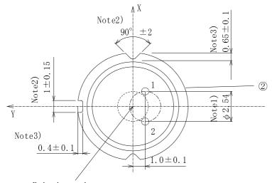
Enlarged drawing around the emission point X↑ Emission point  $0 \pm 0.08$  $0 \pm 0.08$
